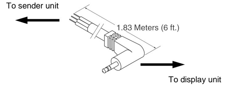
The link cable connects the sender unit to the display unit. The cable should be connected to the sender unit as described in the table below.
