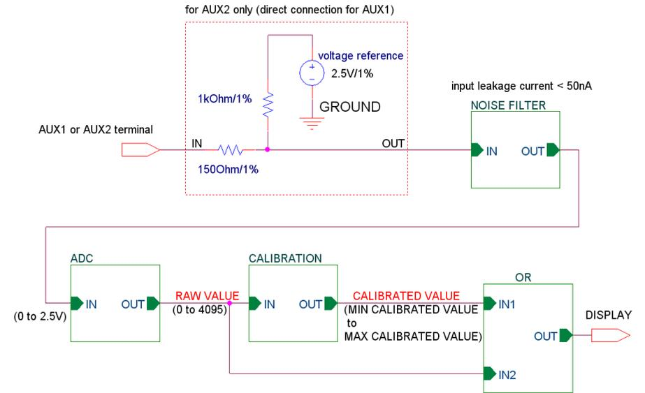
Figure 1 – AUX inputs block diagram
